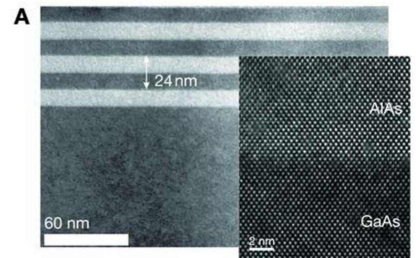
Artificial multilayers (GaAs/AlGaAs)  $\approx 8\text{-}30 \text{ MW/m}^2\text{K}$
