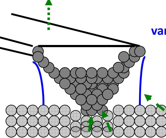
**Amplitude modulation AFM (tapping mode AFM):**
