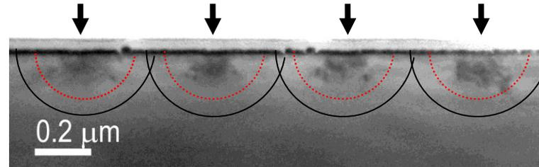
Local anisotropic strain in the zones beneath the indentation lines
