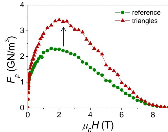
Vortex pinning assigned to the local spatial thickness modulation → Reduction of the vortex line free energy
