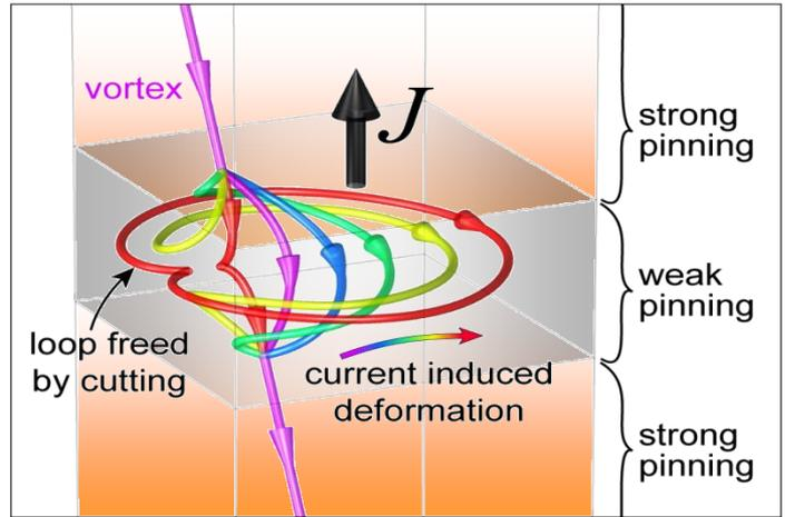
well controlled weak pinning channels →
