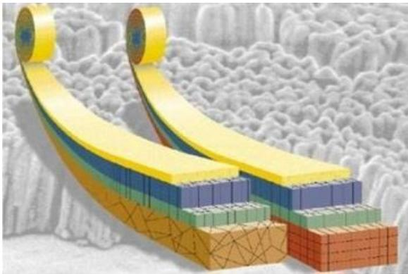
Km length epitaxial multilayer carrying more than 150 times higher current density than Cu
