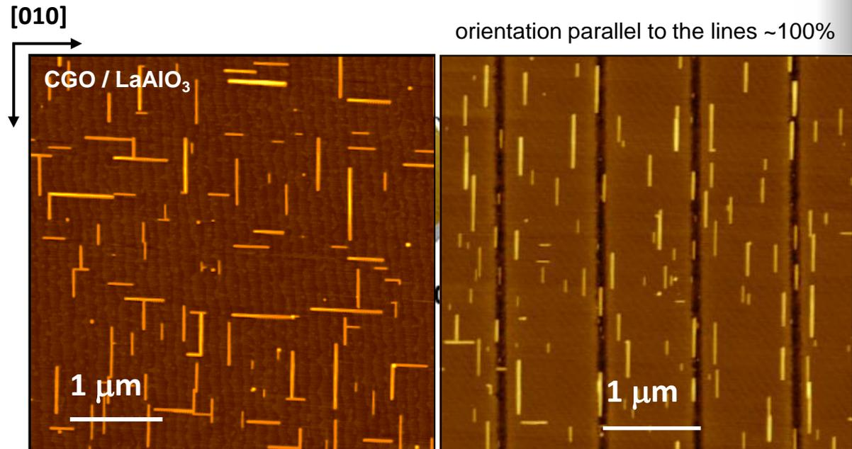
local anisotropic strain → breaking of the pre-existing orientation degeneracy
