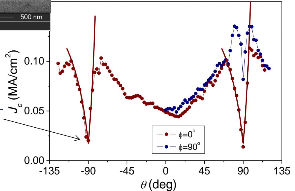
Easy vortex flow along the *ab* – planes → vortex cutting and channeling
