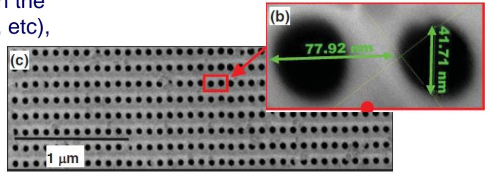
nanoperforated PMMA layer used as a mask through which O+ ions are irradiated
