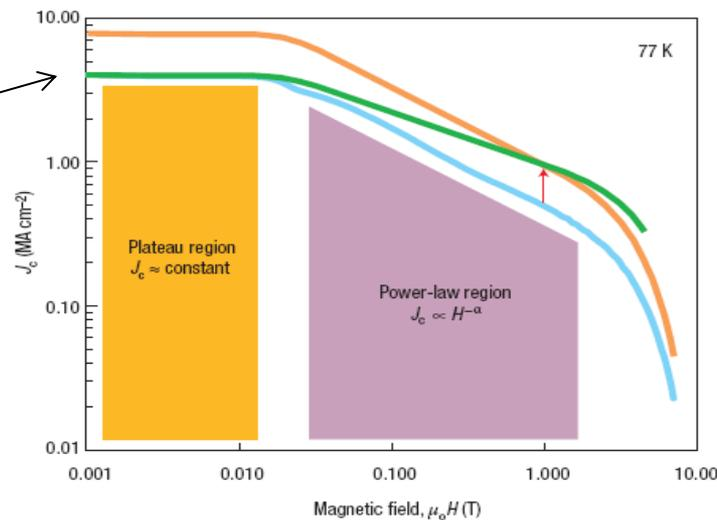
**Nanotechnology:** Essential tool for superconducting applications → Introduce artificial vortex pinning defects to improve  $J_c$  at high fields
