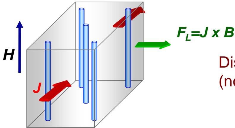
Dissipation due to vortex motion
