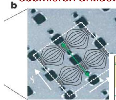
Double antidot array → asymmetric pinning potential
