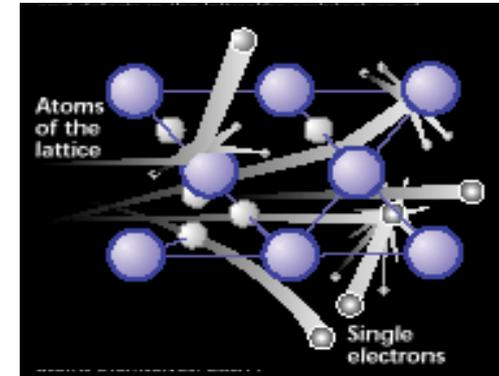
Electrical resistance due to collisions
