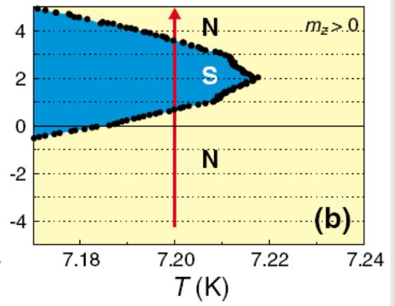
Magnetic-field-induced superconductivity due to the compensation of the applied field by the stray field of the dipoles.
