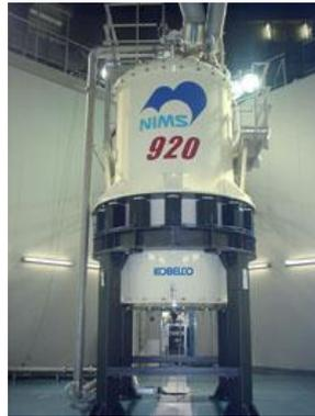
Very high magnetic fields combining first and second generation wires (>23 T 1 GHz)
