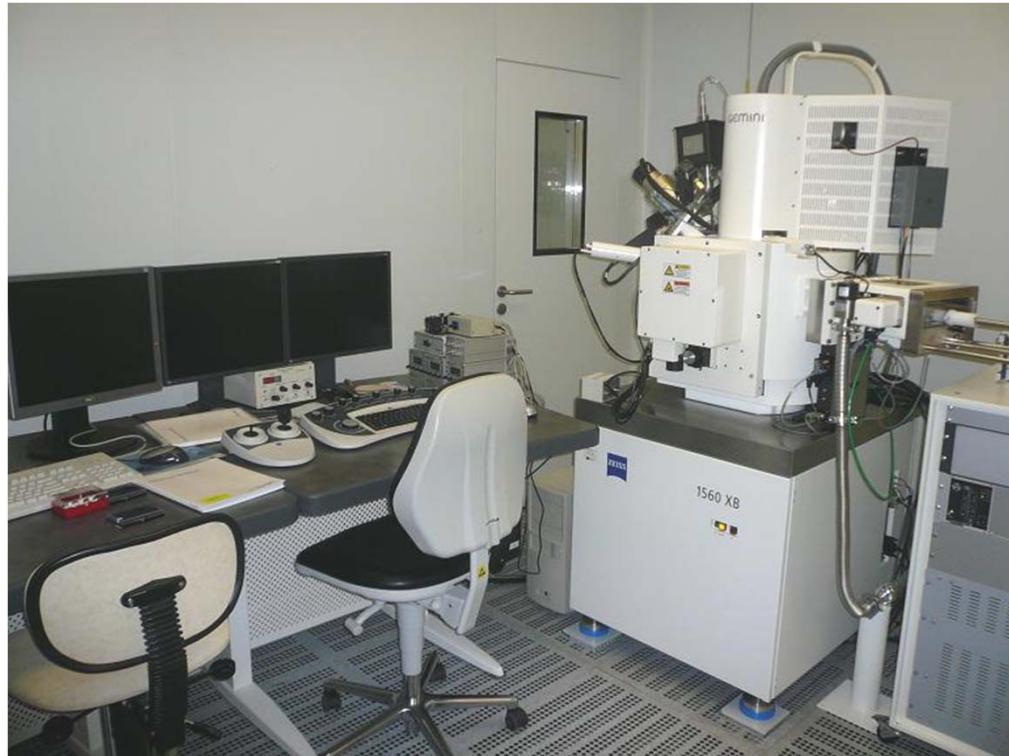
**CROSS BEAM:** Combination of electron and ion columns which allows “real-time” SEM monitoring of FIB modifications
