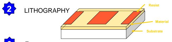
3 ETCHING + RESIST REMOVING Material Substrate
