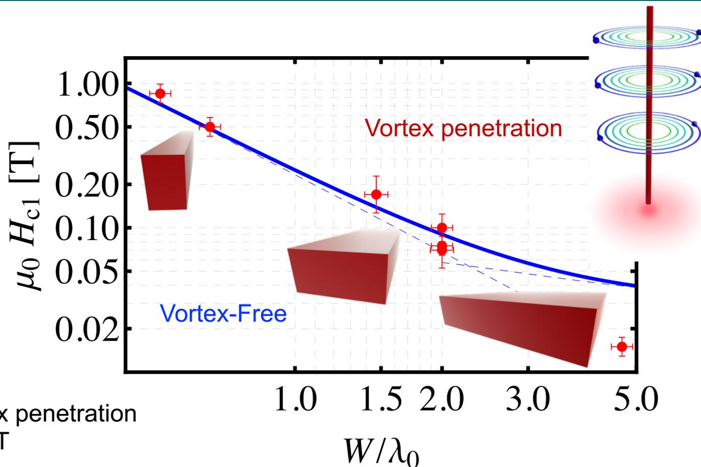
For widths  $W$  much smaller than  $\lambda$  vortex penetration field can reach values on the order of 1 T
