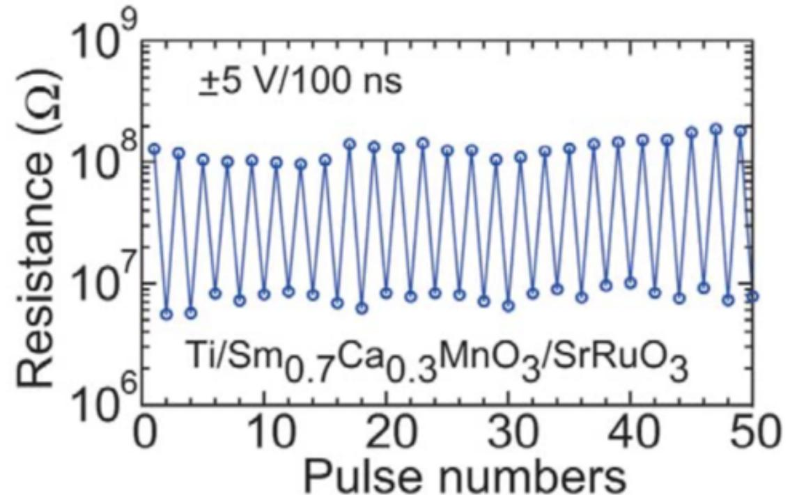
large change in resistance ( $>1000\%$ ) on applying pulsed voltages
