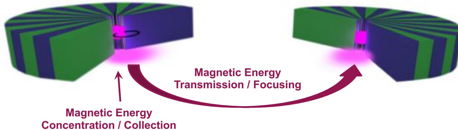
Use metamaterial shells composed of concentric pieces made of FM-SC for **guiding, concentrating, harvesting, and transferring static and low-frequency magnetic fields, at micro- / nano-scale**
