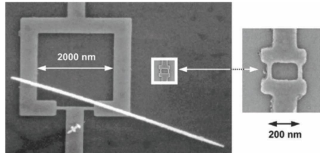
Nb microSQUID & nanoSQUID fabricated by EBL
