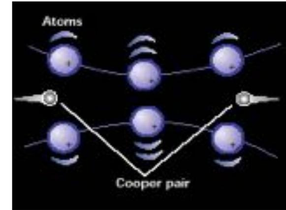
Electrical conduction via Cooper pairs
