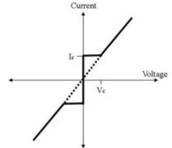
Cooper pairs can electrically tunnel across two superconductors separated by a thin insulating or normal metal barrier
