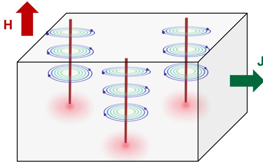
$J_c$ , Critical current density  $\ll$  Depairing current (cooper pair breaking)
