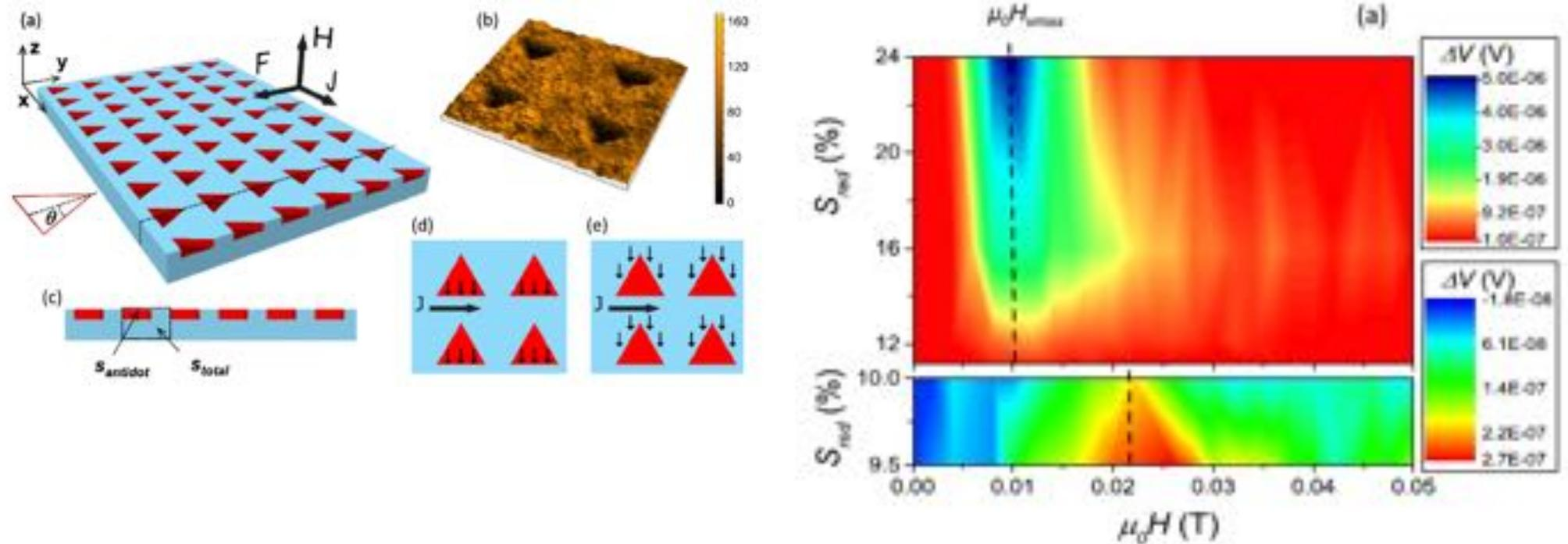
Rectified flux motion arising from the collective effect of many interacting vortices is obtained in a specially designed superconducting device.
