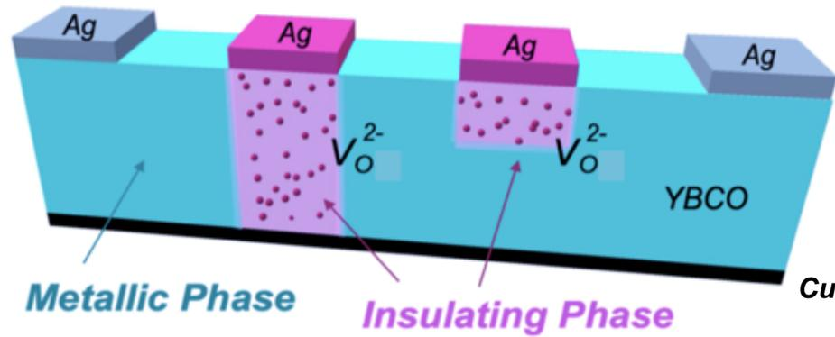
Movement of oxygen ions can mimic the flux of sodium and potassium ions in neurons.
