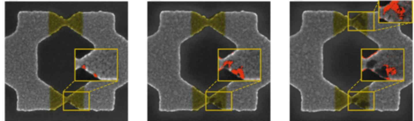
Shrinking of the constriction due to subsequent electromigration processes
