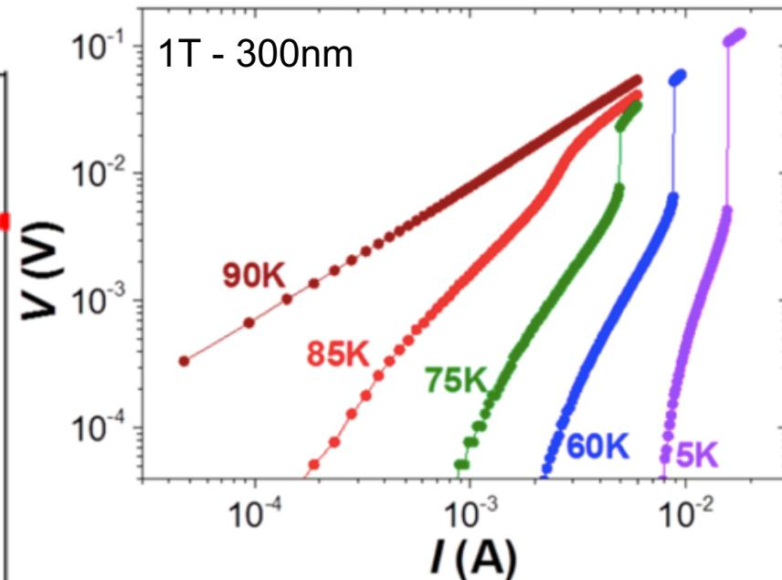
Flux-flow penetration induces very sharp voltage transitions from the superconducting to the normal state → Potential for detector applications
