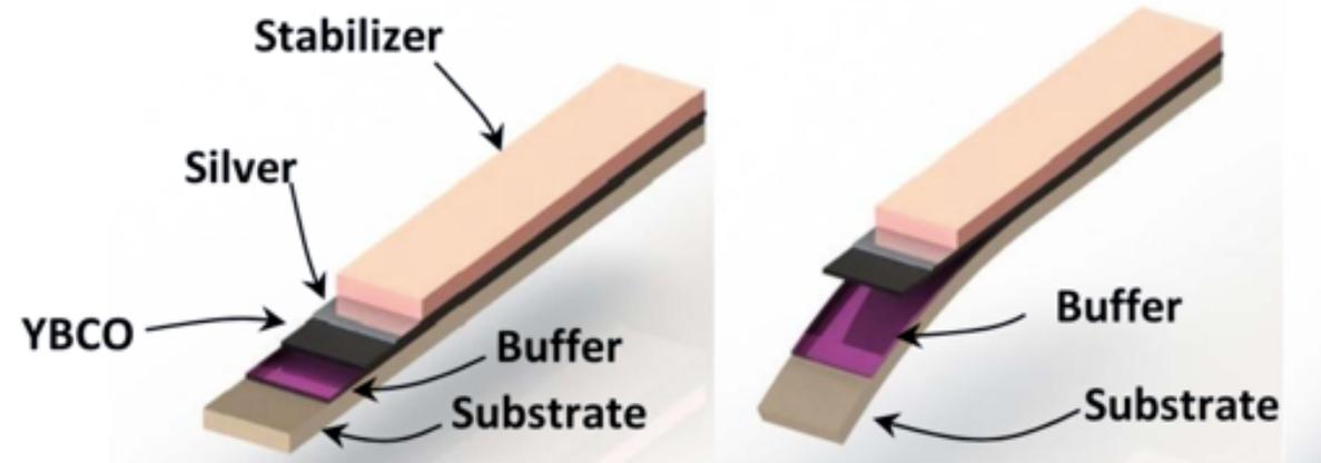
Exfoliation by mechanically stretching the flexible metallic tape
