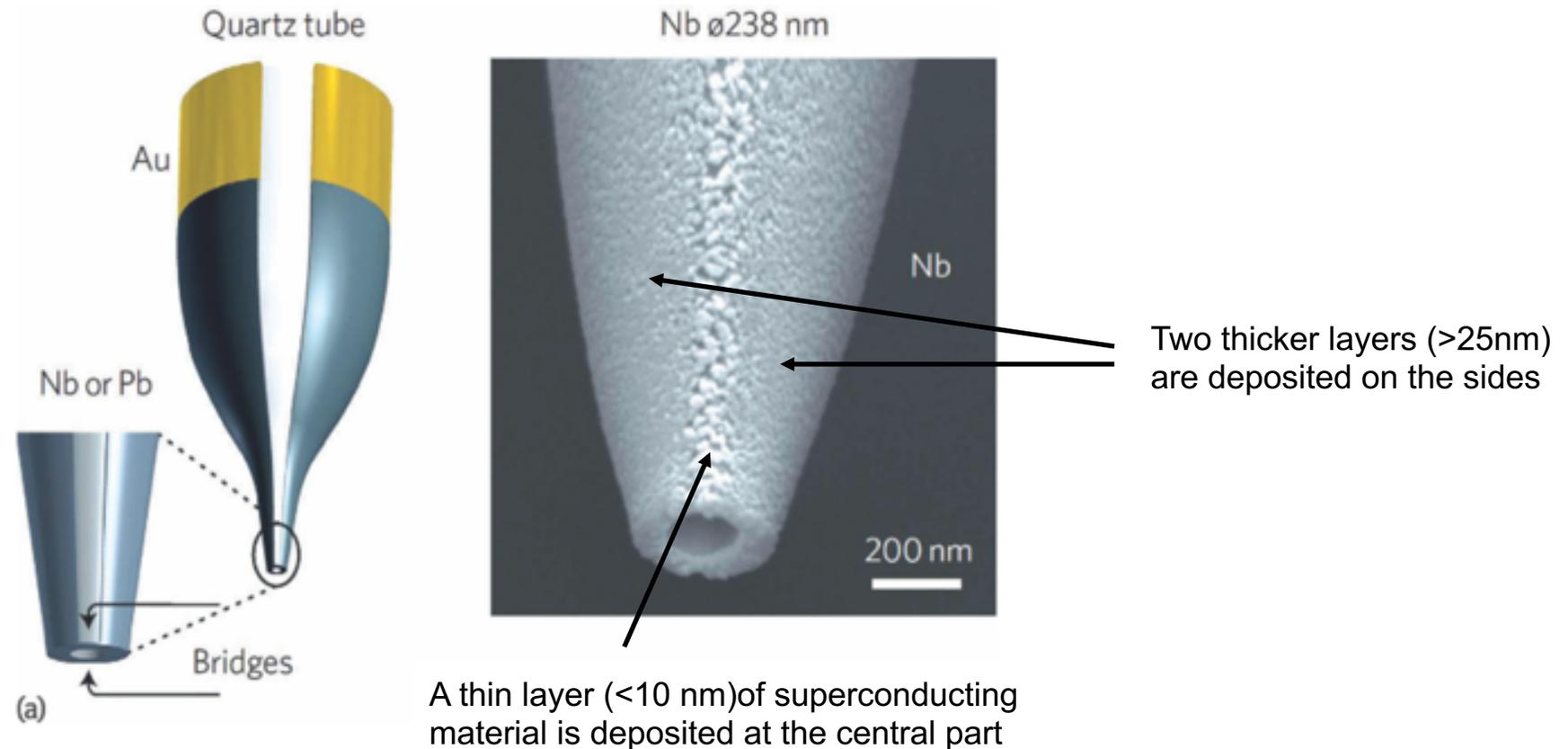
This procedure lead to the smallest nanoSQUIDs fabricated so far, with effective nano-loop diameters down to 50 nm
