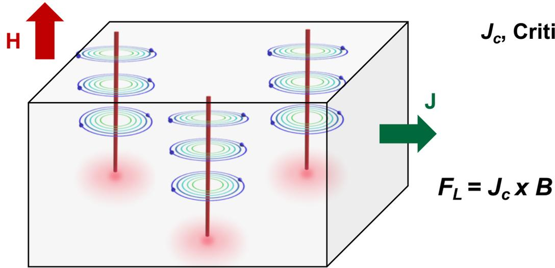
$J_c$ , Critical current density  $\ll$  Depairing current (cooper pair breaking)
