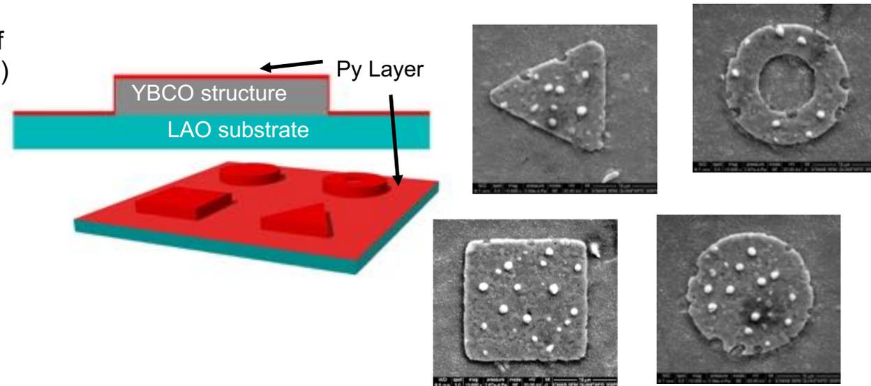
→ Flux penetration / distribution completely depends on the **sample geometry**
