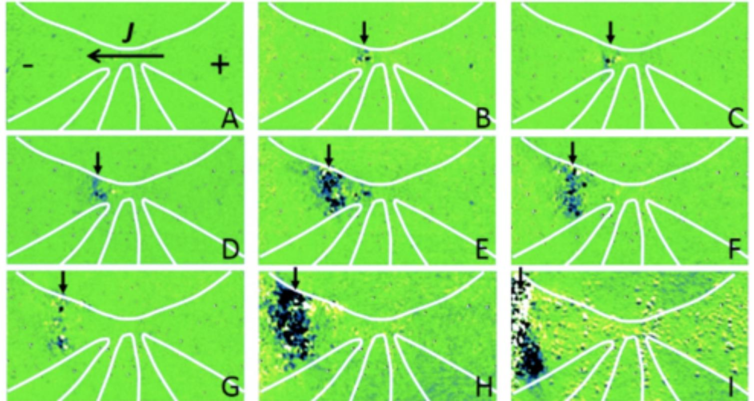
Oxygen vacancy displacement towards the cathode (-) visible by optical microscopy
