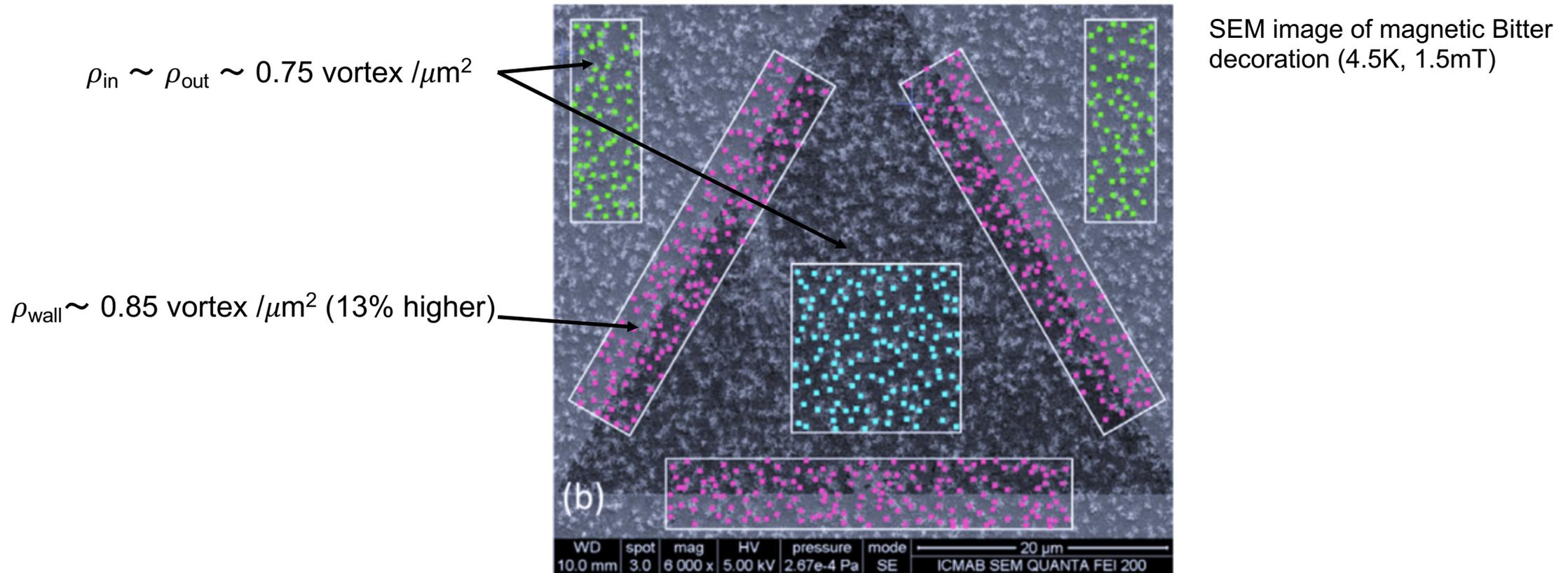
Nanowalls are acting as very effective pinning sites → Reduction of the order parameter near the nanowalls by localized deoxygenation or amorphization of the YBCO structure
