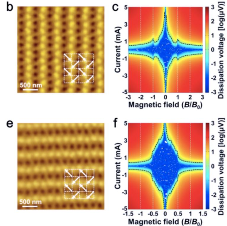
The tuneable magnetic charges in the artificial-spin-ice strongly interact with the flux quanta in the superconductor
