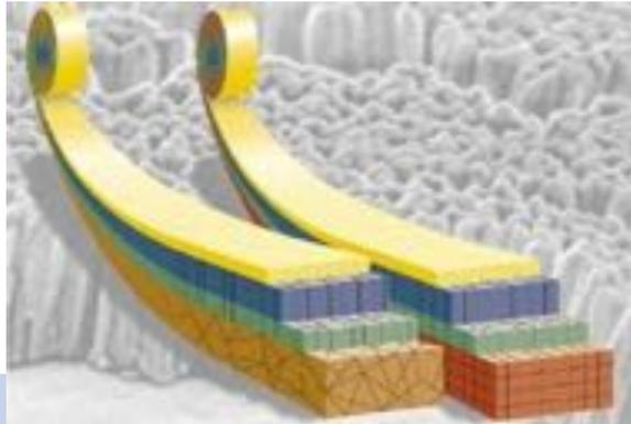
Textured YBCO film exfoliated from a metallic substrate that can be transferred onto the desired substrate
