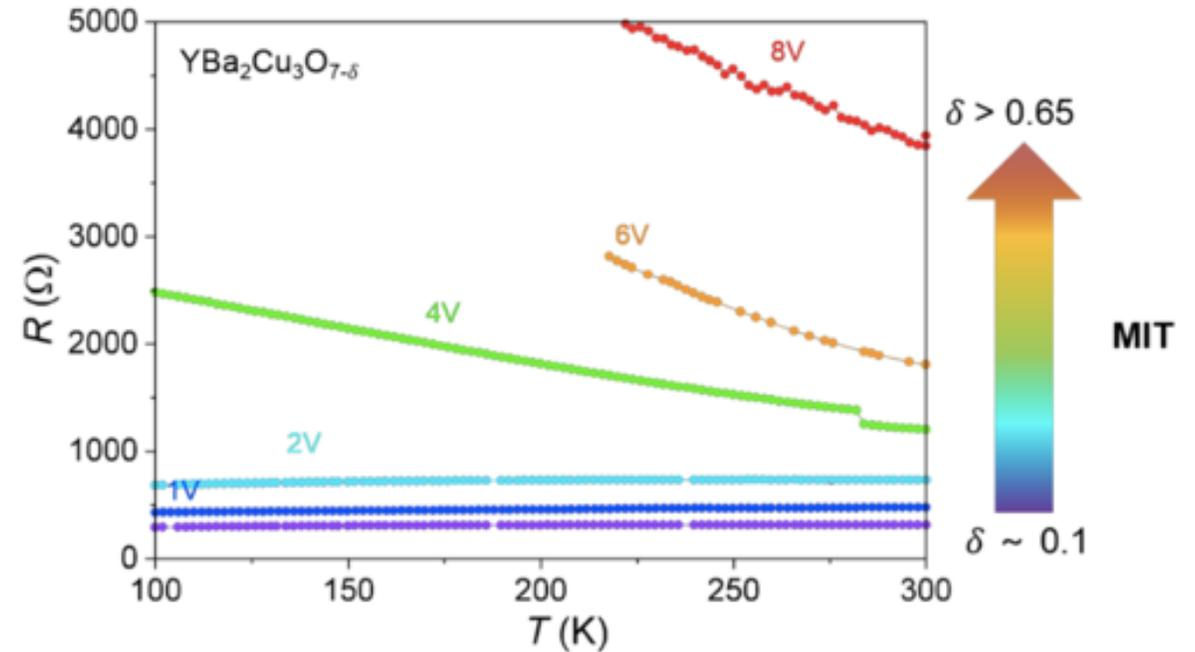
**Field-induced reversible robust volume Metallic to Insulator Transition (MIT) through oxygen doping:**
