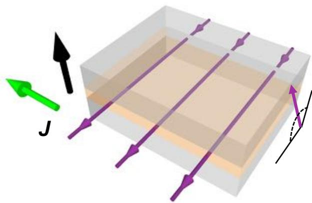
Easy vortex flow along the  $ab$  – planes → vortex cutting and channelling
