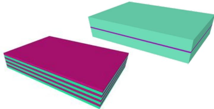
Vortex motion along layers with different pinning →
