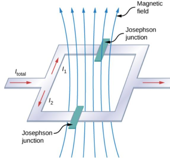
SQUIDs combine the Josephson effect with the quantization of magnetic flux in superconductors
