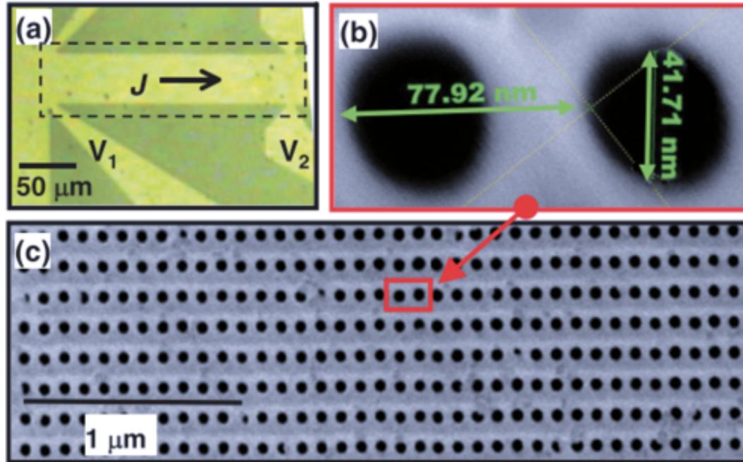
Holes of  $D \sim 40\text{nm}$  with inter-hole distance  $d \sim 120\text{ nm}$
