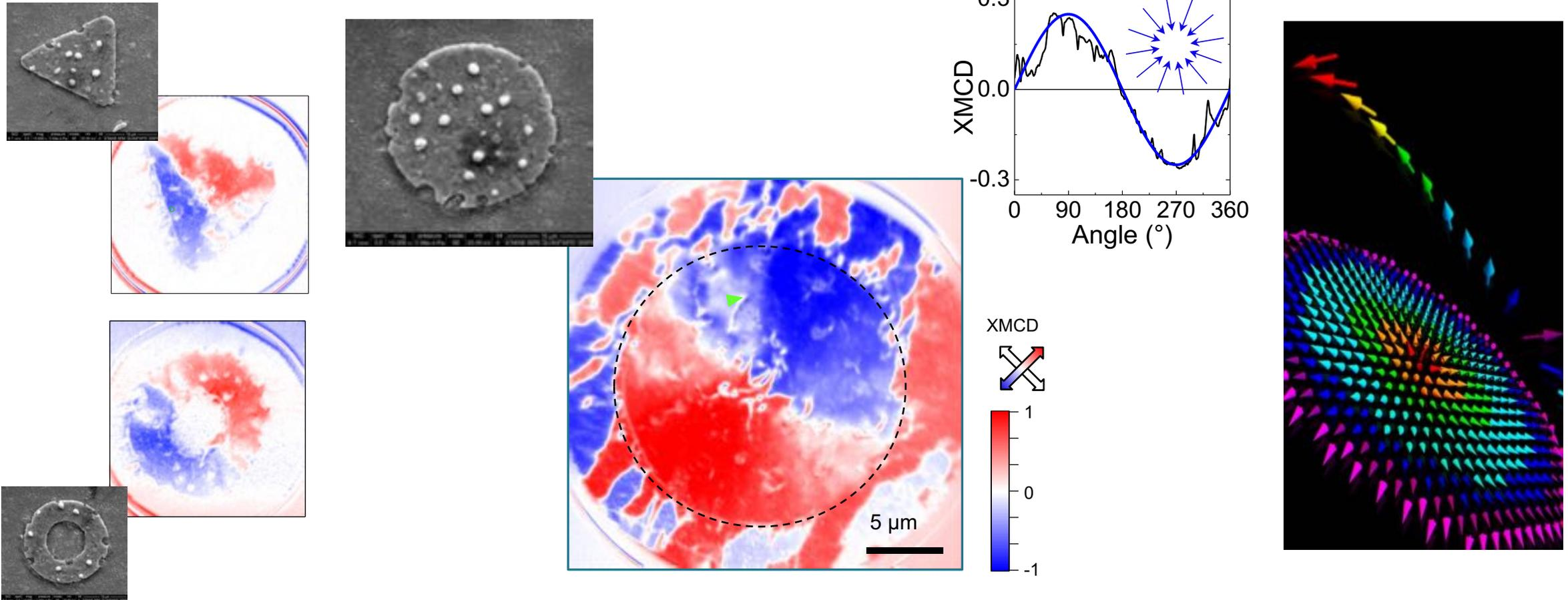
**2D monopole-like spin texture** configuration, whose magnetic charge can be easily switched from +1 to -1 by changing the sign of  $B_{\max}$
