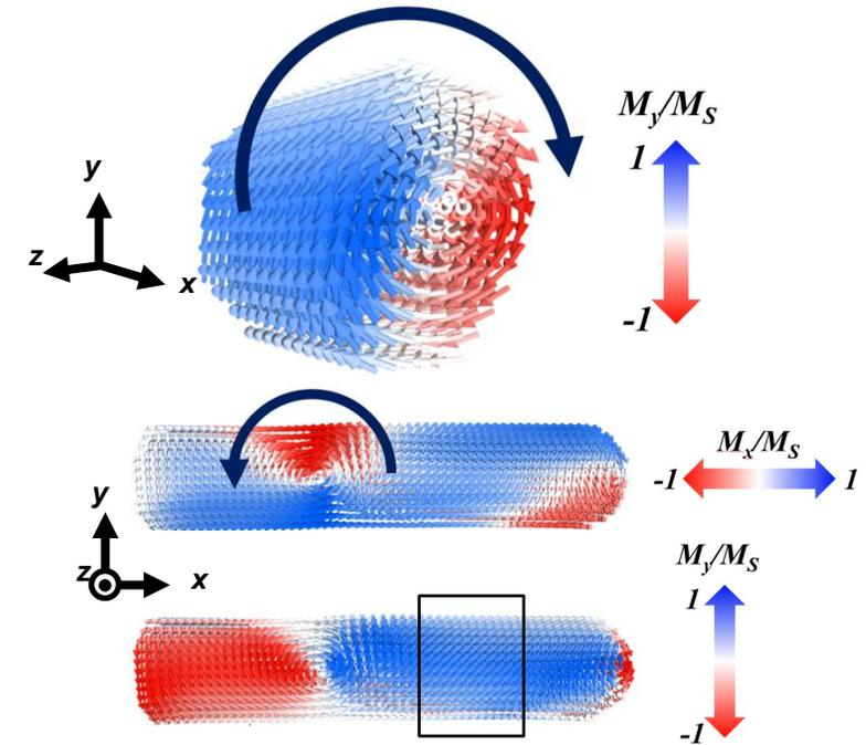
SC properties of the film and 3D nanometric magnetic structure of the Co nano-rods tuned by cooperative non homogenous SC-FM stray fields.
