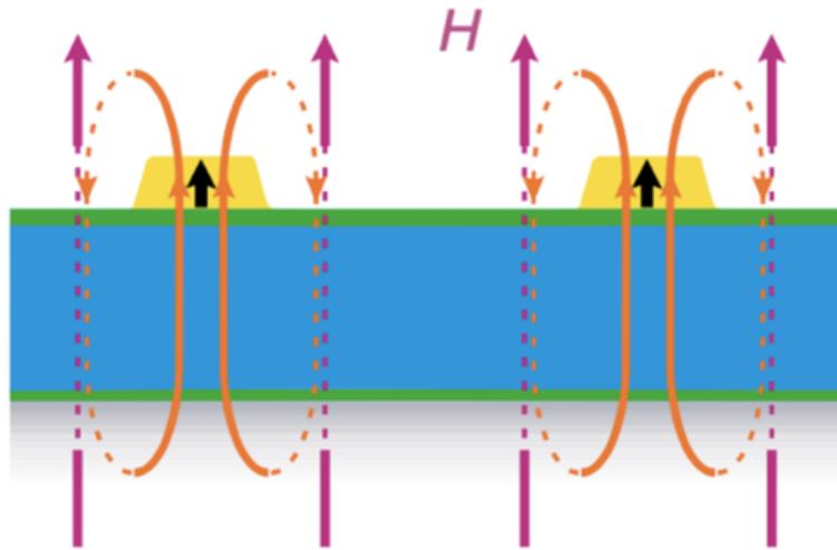
Superconducting Vortices may act as tiny Magnetic Tweezers to modify magnetic spins
