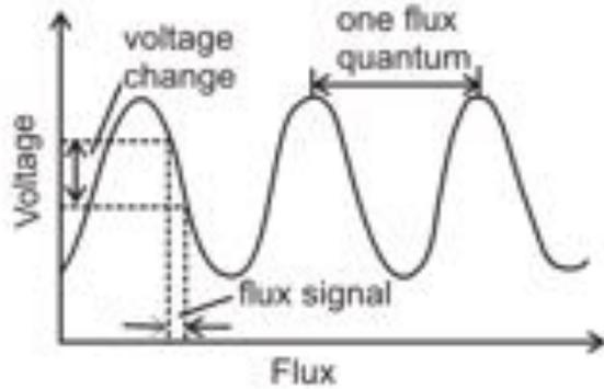
Large voltage changes associated with one flux quantum
