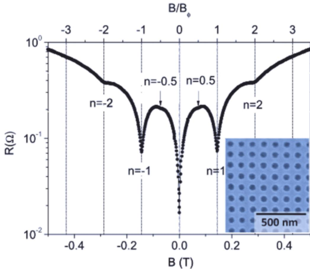
Nanometric distances  $\rightarrow$  vortex manipulation in very high magnetic fields (up to two orders of magnitude higher than with other techniques)
