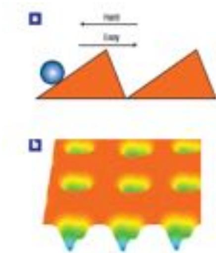
Ratchet effects in superconducting systems → size and quantity of particles (vortices) can be finely tuned with two external parameters ( $T$  and  $H$ )
