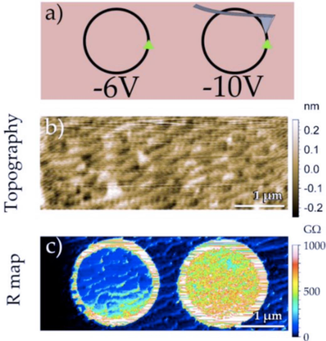
Conducting AFM → control over the metal-insulator transition at nanometric scales
