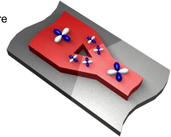
Although micrometric SQUIDs based on GBJs have been successfully produced the miniaturization of high-quality GBJs is challenging, because of degradation of the material due to oxygen loss during nanopatterning
