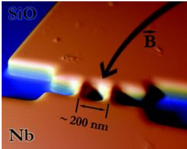
Nb nanobridges (80nm) fabricated by FIB
