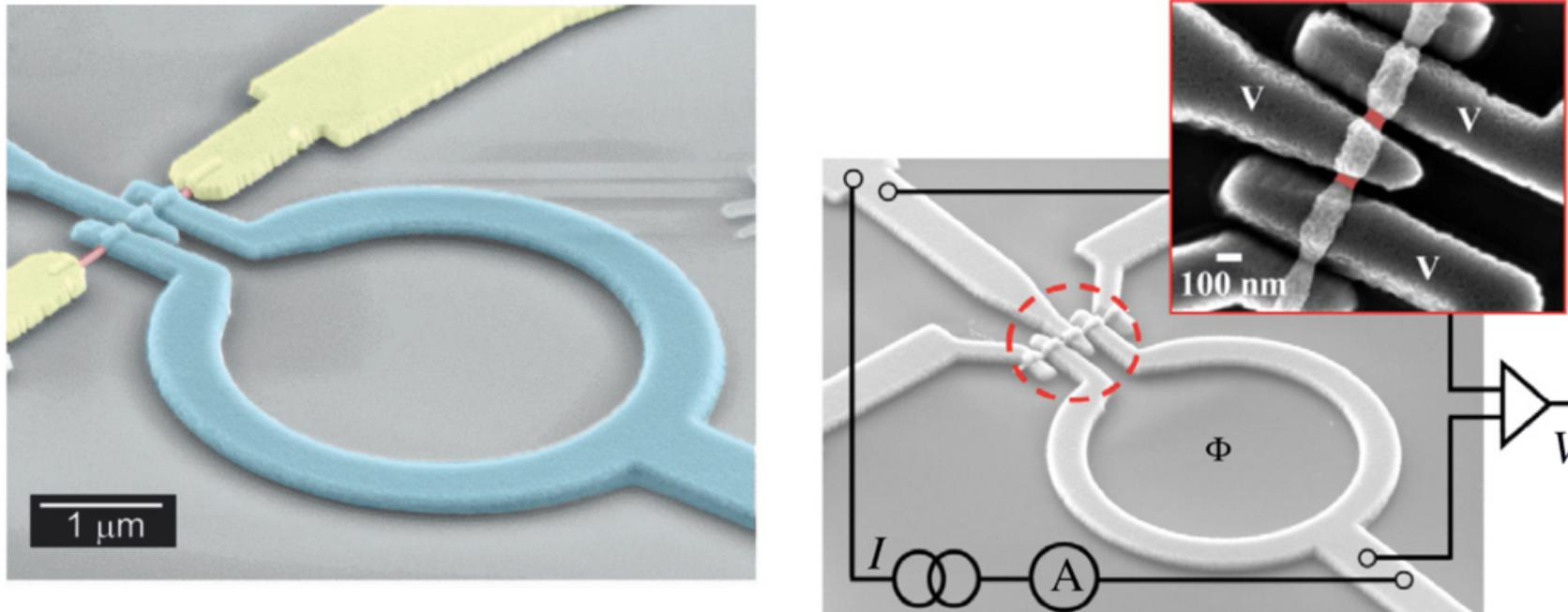
weak link between vanadium (V) superconducting electrodes and an indium arsenide (InAs) nanowire
