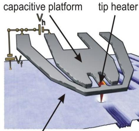
Thermal sensor for height signal
