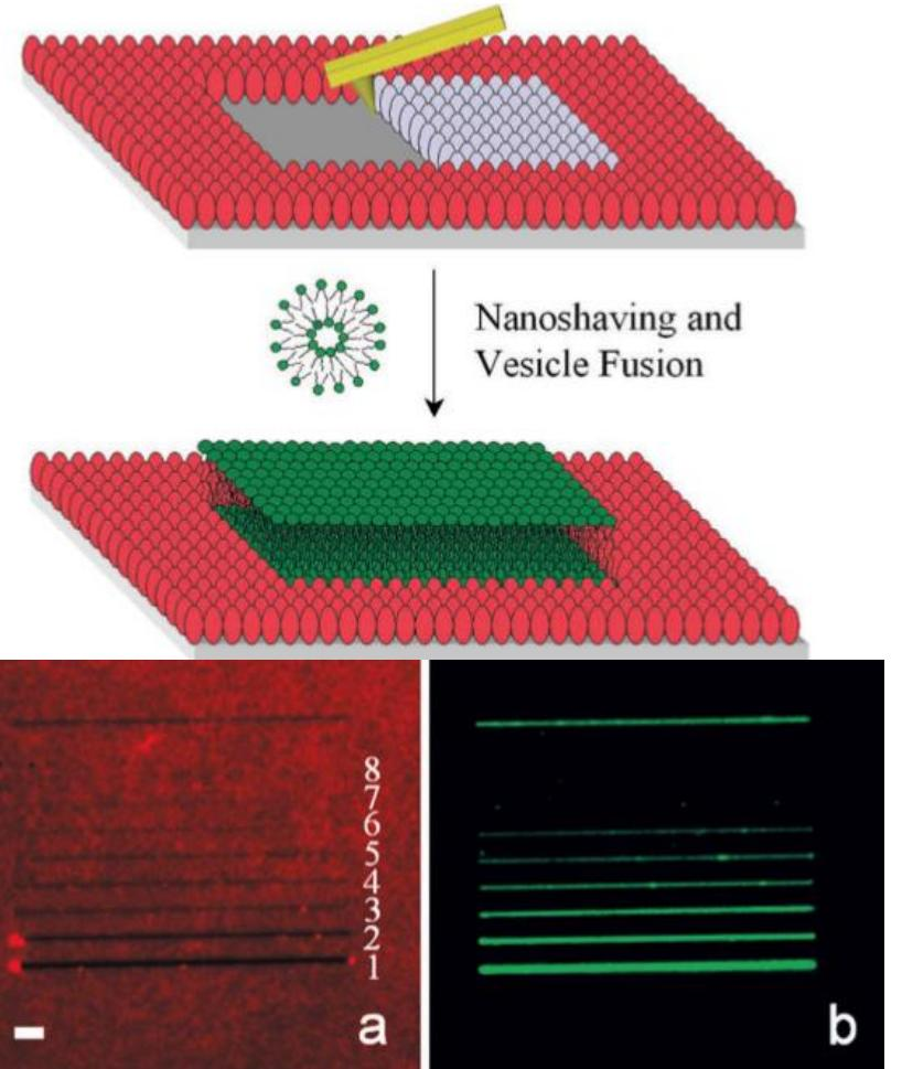
Epifluorescence images of (a) a nanoshaved BSA monolayer and (b) SLB lines. The top line, which is ~200 nm in width, was used as a reference marker
