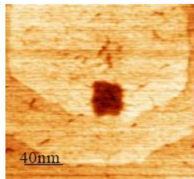
CH<sub>3</sub>-(CH<sub>2</sub>)<sub>9</sub>-SH nanografted into a CH<sub>3</sub>-(CH<sub>2</sub>)<sub>17</sub>-SH SAM (400 Å × 400 Å)
