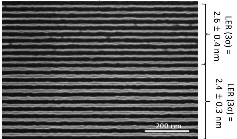
STEM cross sections from one of the arrays of 14 nm half-pitch SiNWs
