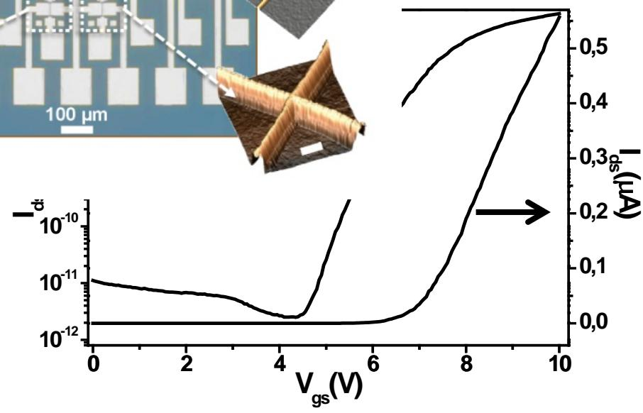
subthreshold swing is close to the theoretical limit for device of this geometry
