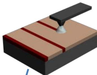
3. PS-*b*-PMMA deposition + Annealing
