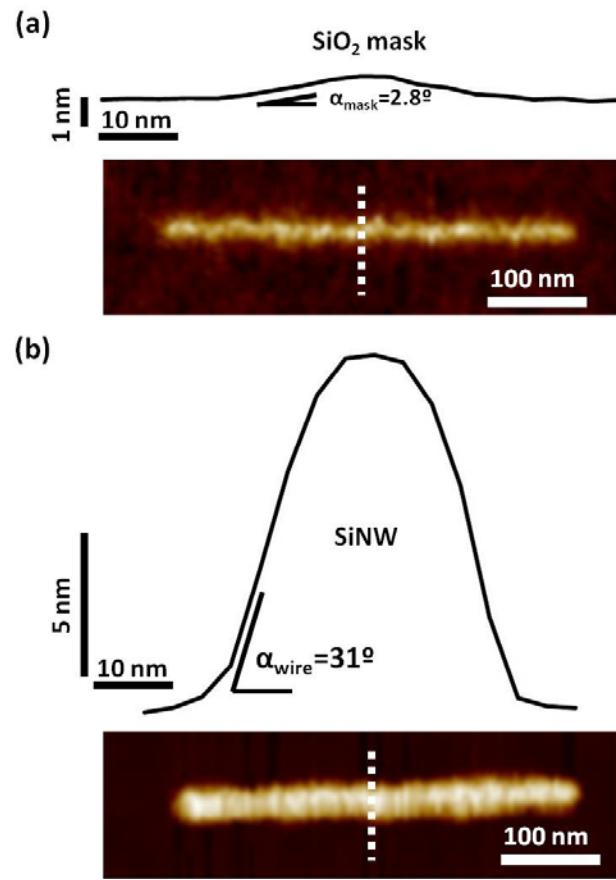
**The oxide mask height is controlled by the voltage amplitude**
