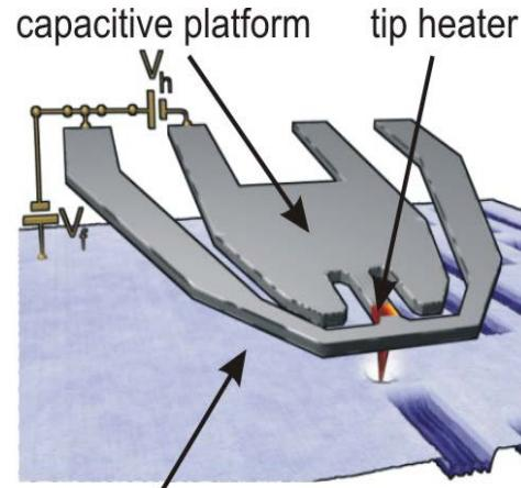
Thermal sensor for height signal
